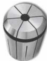
HP - High Precision Collet (.0002"/5 micron TIR) (.020/.5mm collapse range)
