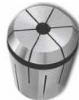
Steel-Sealed Coolant Collet 1000 PSI - 0.0004"/10 micron TIR (no collapse range)
